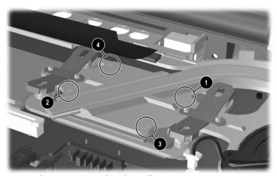
Heat Sink Screw Removal and Installation Sequence
